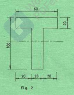
(b) Calculate the moment of resistance of the beam section if the stresses in upper and lower sections are limited to 10 N/mm² and 25 N/mm² respectively. (5 marks)
